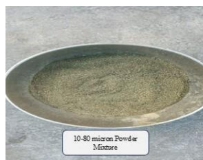
Figure 8. Grounded AP powder mixture of (10-80μ)
