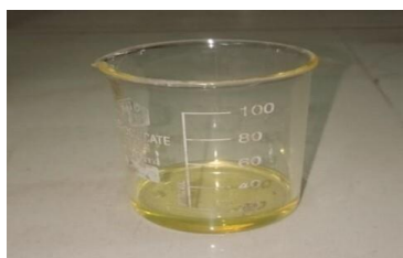
Figure 23. Oil Got from 50% Dried (10-80) Micron AP Powder Mixture
