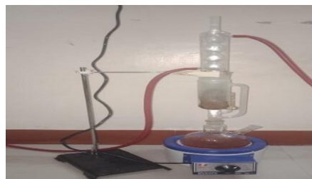
Figure 15. 1-litre capacity of Soxhlet Extraction kit
