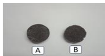
Figure 9. Test Samples for Microscope (a) 0.5-10 Micron Powder, (b) 10-80 Micron Powder
