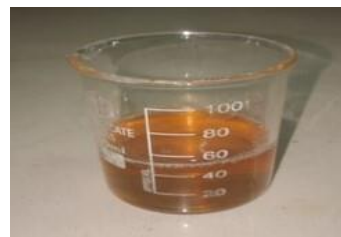
Figure 29. Oil Got from 100% Dried (0.5-10) Micron AP Powder Mixture
