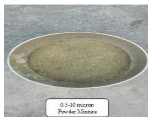
Figure 7. Grounded AP powder mixture of (0.5-10μ).
