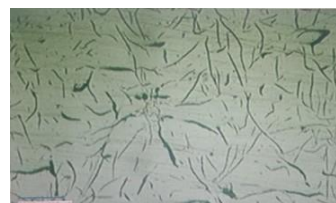
Figure 11. Microscopic view of (10-80) Micron Mixture AP Powder Size
