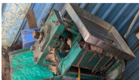
Figure 6. Oil Extraction mechanical presser.
