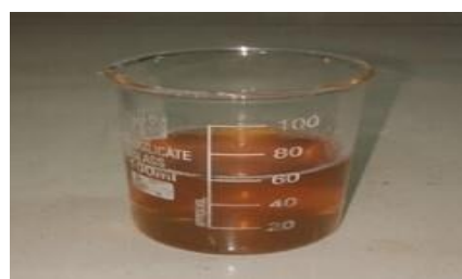
Figure 31. Oil Got from 100% Dried (0.5-10) Micron AP Powder Mixture
