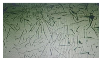
Figure 10. Microscopic view of (0.5-10) Micron Mixture AP Powder Size
