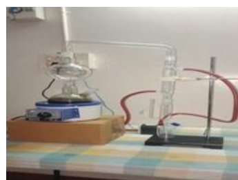
Figure 13. One liter capacity of Steam Distillation extraction apparatus
