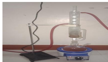
Figure 15. 1-litre capacity of Soxhlet Extraction kit
