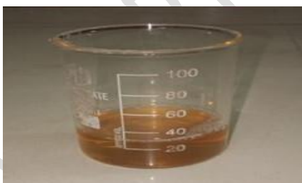
Fig. 30. Oil Got from 50% Dried (0.5-10) Micron AP Powder Mixture
