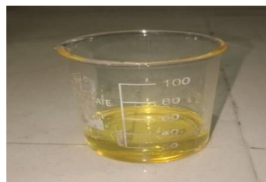
Fig. 24. Oil Got from 100% Dried (10-80) Micron AP Powder Mixture
