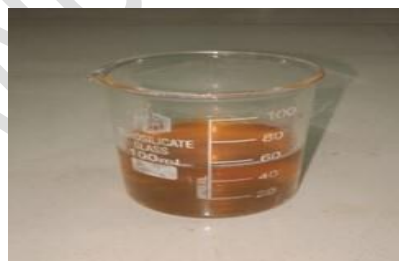
Fig. 33. Oil Got from 100% Dried (0.5-10) Micron AP Powder Mixture
