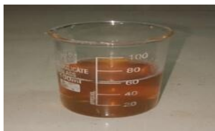
Fig. 31. Oil Got from 100% Dried (0.5-10) Micron AP Powder Mixture
