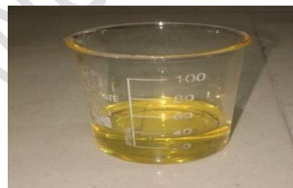
Fig. 26. Oil Got from 100% Dried (0.5-10) Micron AP Powder Mixture
