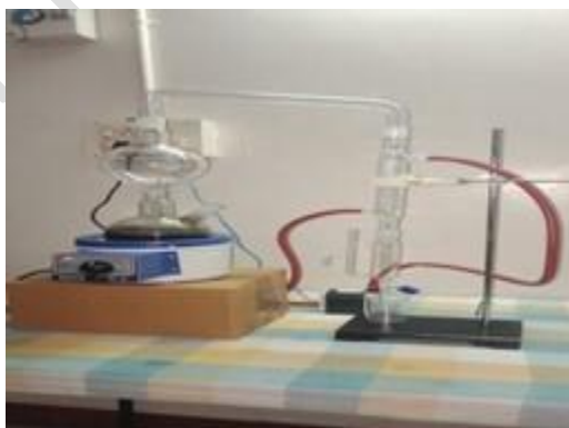
Fig. 13. One liter capacity of Steam Distillation extraction apparatus
