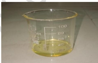
Fig. 23. Oil Got from 50% Dried (10-80) Micron AP Powder Mixture
