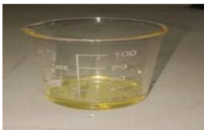
Fig. 25. Oil Got from 50% Dried (0.5-10) Micron AP Powder Mixture
