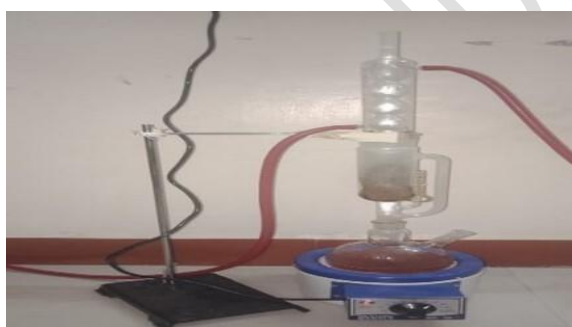
Fig. 15. 1-litre capacity of Soxhlet Extraction kit
