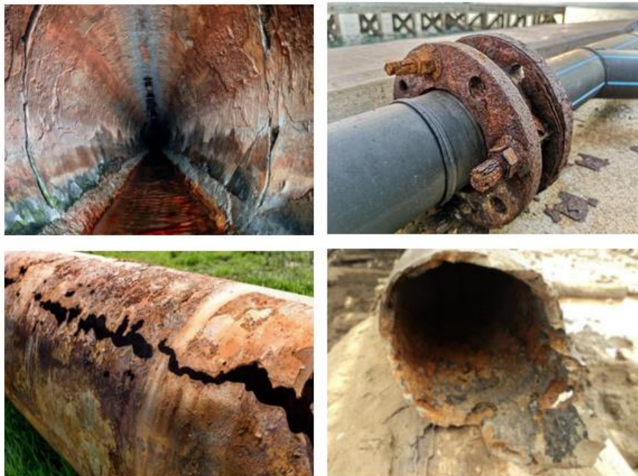
Figure 1. Corroded and eroded sewage pipes, drains and couplings due to toxic gases
