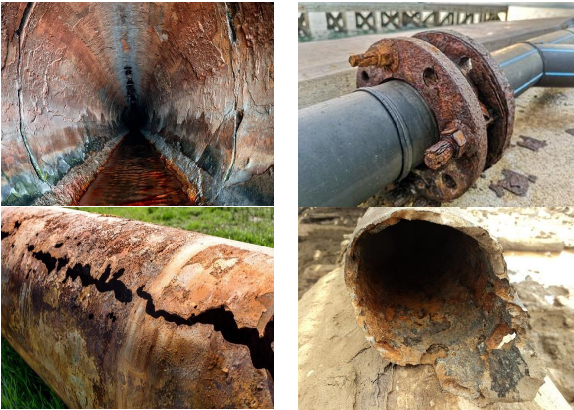
Fig.1. Corroded and eroded sewage pipes, drains and couplings due to toxic gases
