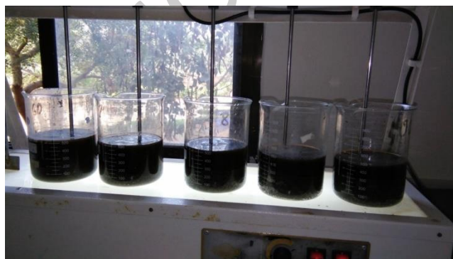
Figure 1. Coagulation process for treating textile effluent
