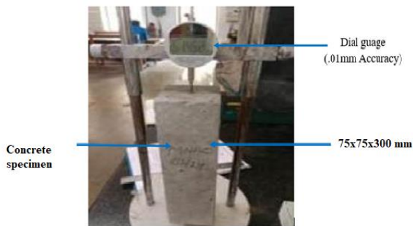
Figure 3. Test setup for Drying Shrinkage
