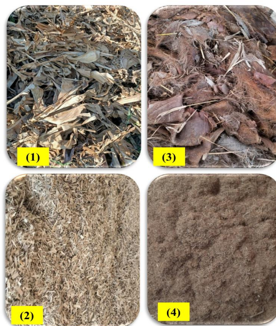
Figure 1. Agro-waste in the form of raw materials of banana leaves and date palm fibers (photos 1 and 3) as well as their crushed forms (photos 2 and 4, respectively)
