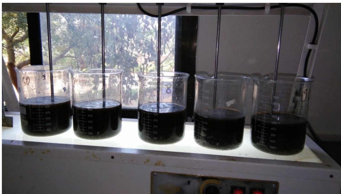
Fig.1 Coagulation process for treating textile effluent
