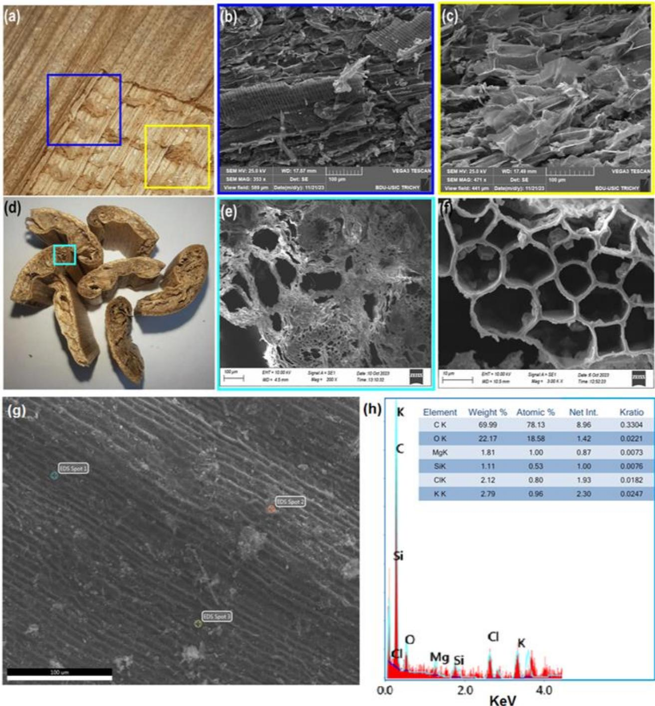
Figure 6. (a) pseudostem sheath (b) and (c) SEM image of pseudostem biochar outer layer and middle layer (d) Sheath's transverse section (e) SEM image of sheath's transverse section (f) SEM image of biochar's transverse section (g) EDSEM image of pseudostem biochar outer layer showing 3 spots and (h) EDS spectrum of spot 2
