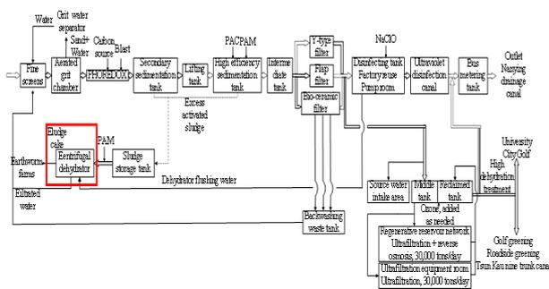
**Figure 2.** Process flow of upgrading and reconstruction project
