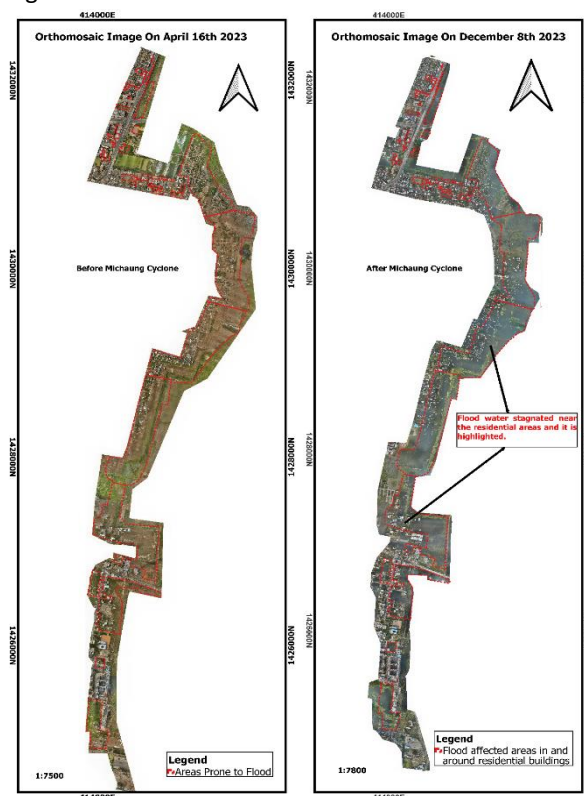
Figure 5: Comparison of Pallikaranai Drone Data using orthomosaic image of Pre-disaster vs Post disaster
