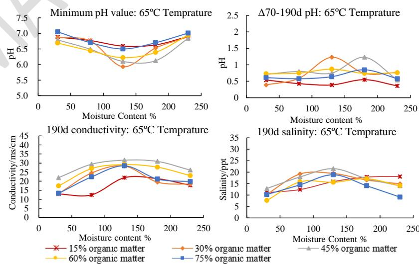
Figure 7. Effect of moisture content on the degradation characteristics of MSW
