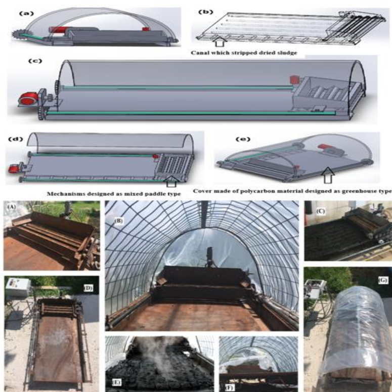
Figure 2. Pilot scale hybrid sludge drying system. (a) side views (b) resistances (c) front views (d) mechanisms designed side by side and like mixer paddle type (e) polycarbonate material that can pass the sun rays easily. (A) The mixer-paddle mechanism of system (B) inside of dryer (C) the moment the dewatered sludge is laid in the dryer (D) electrical resistances (E) drying sequence (F) the appearances of the sludge in the drying area (G) external view of the system
