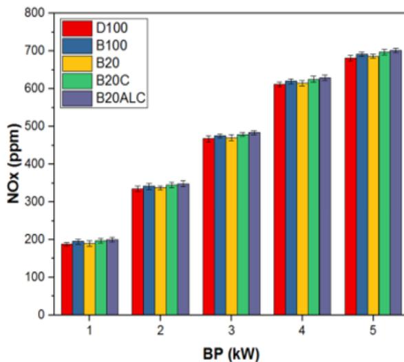
**Figure 10.** Nitrogen oxide outcomes of diesel engine functioned with terminalia catappa seed oil mixed with alumina nanoparticles
