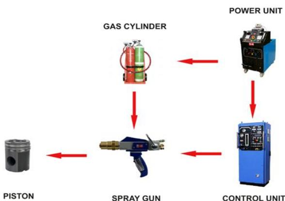
**Figure 3(a).** Thermal barrier coating process
