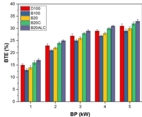
**Figure 6.** BTE outcomes of diesel engine functioned with terminalia catappa seed oil mixed with alumina nanoparticles
