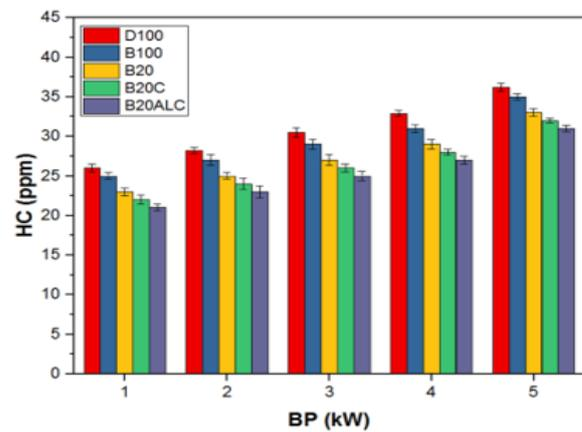
**Figure 8.** HC outcomes of diesel engine functioned with terminalia catappa seed oil mixed with alumina nanoparticles
