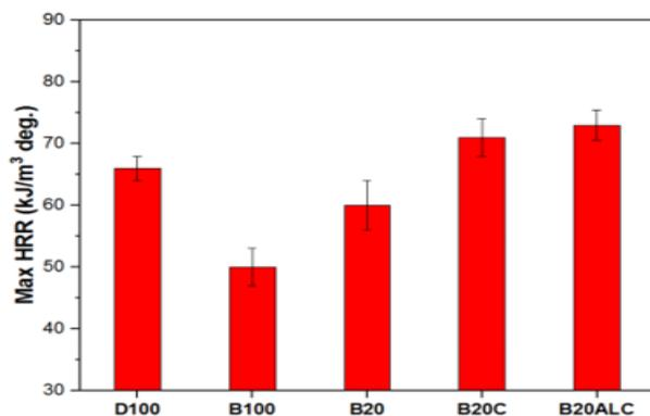
**Figure 12.** Maximum heat release rate outcomes of diesel engine functioned with terminalia catappa seed oil mixed with alumina nanoparticles
