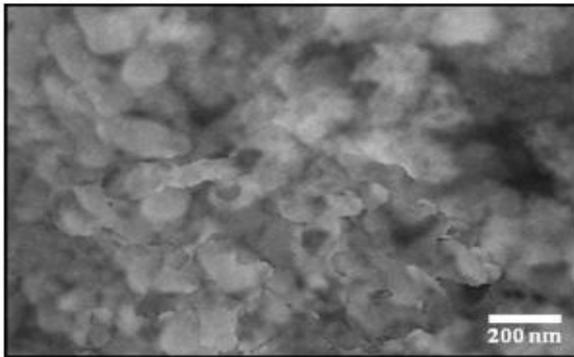
**Figure 2** SEM image of alumina nanoparticles
