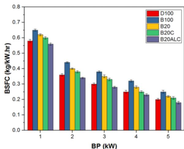
**Figure 5.** BSFC outcomes of diesel engine functioned with terminalia catappa seed oil mixed with alumina nanoparticles
