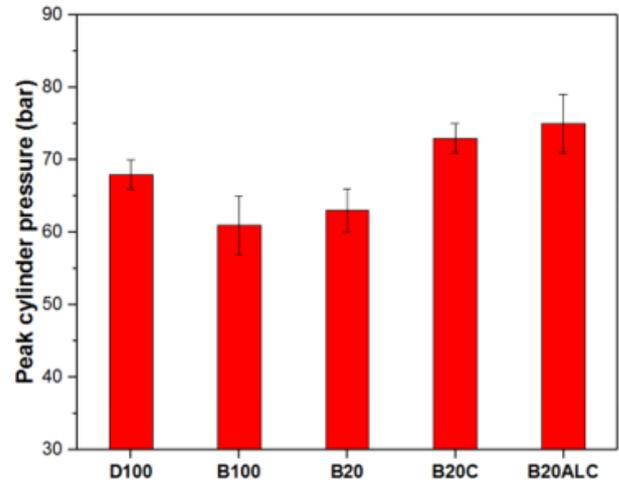
**Figure 11.** Peak cylinder pressure outcomes of diesel engine functioned with terminalia catappa seed oil mixed with alumina nanoparticles
