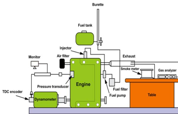
**Figure 4(a).** Schematic representation of experimental setup
