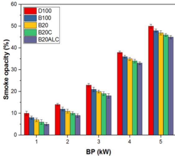
**Figure 9.** Smoke opacity outcomes of diesel engine functioned with terminalia catappa seed oil mixed with alumina nanoparticles
