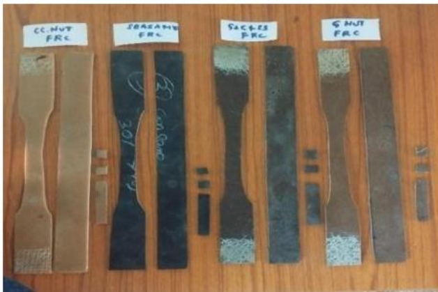
Figure 5. Specimens in ASTM D638 standard
