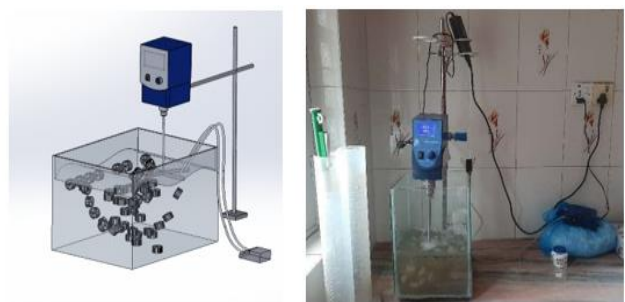
Figure 2. Experimental set-up of MBBR: A. 3D diagram of the reactor B. Actual set-up of the reactor
