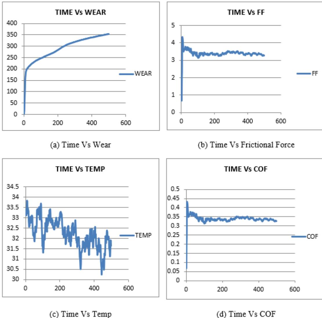
Figure 9. Time-dependent wear test results for SOR sample
