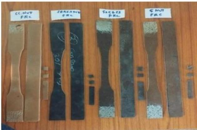
**Figure 5.** Specimens in ASTM D638 standard
