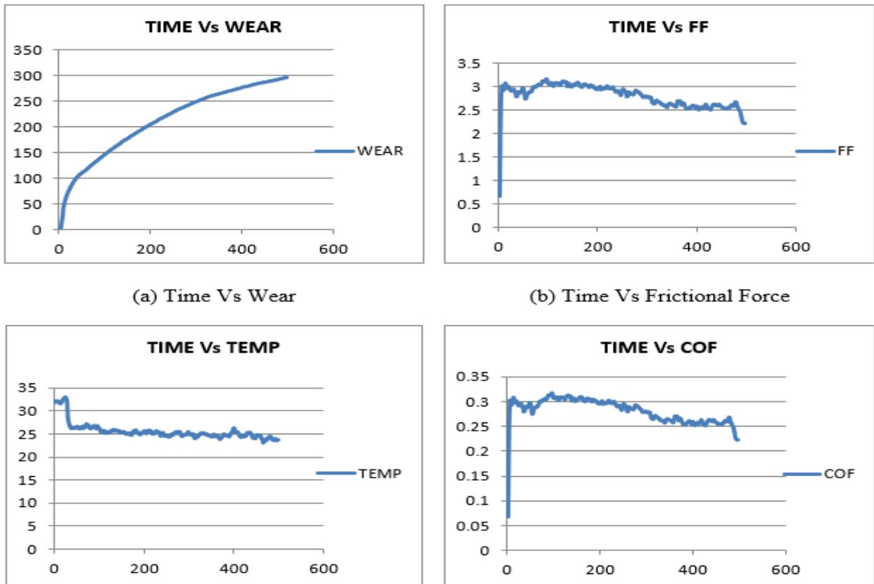
**Figure 10.** Time-dependent wear test results for CGS sample
