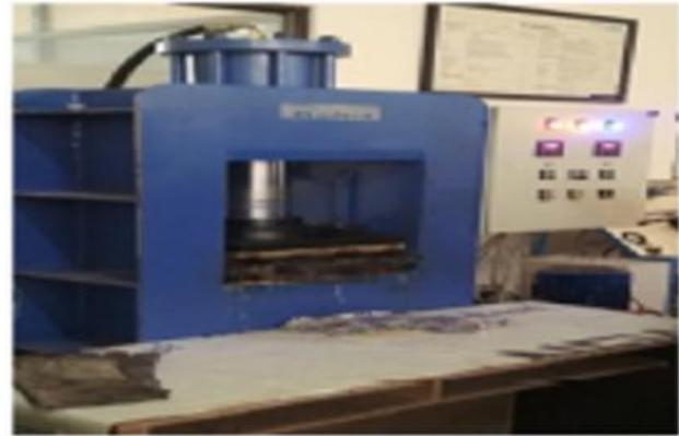
**Figure 2.** Compression molding
