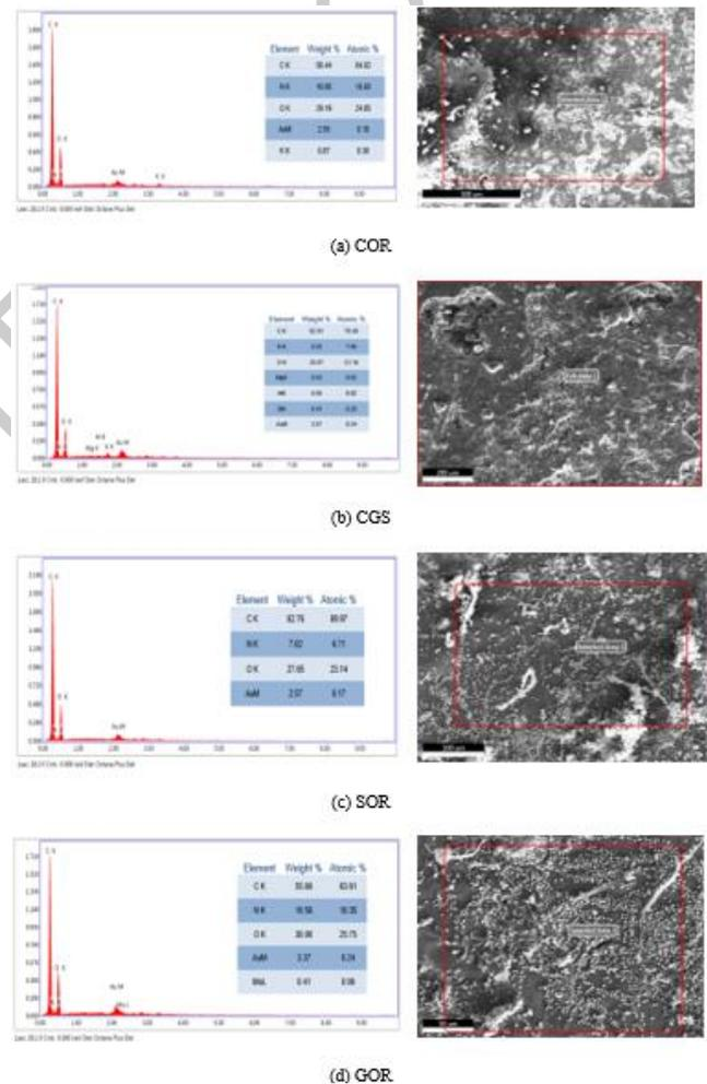
**Figure 15.** EDX analysis of various oil residue compounds.
