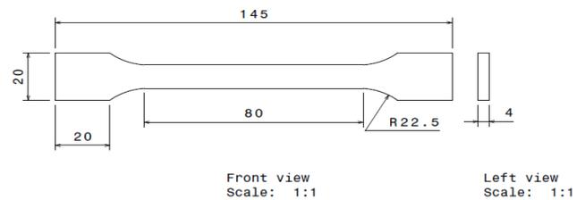
**Figure 4.** Dimensions with ASTM D638 standard
