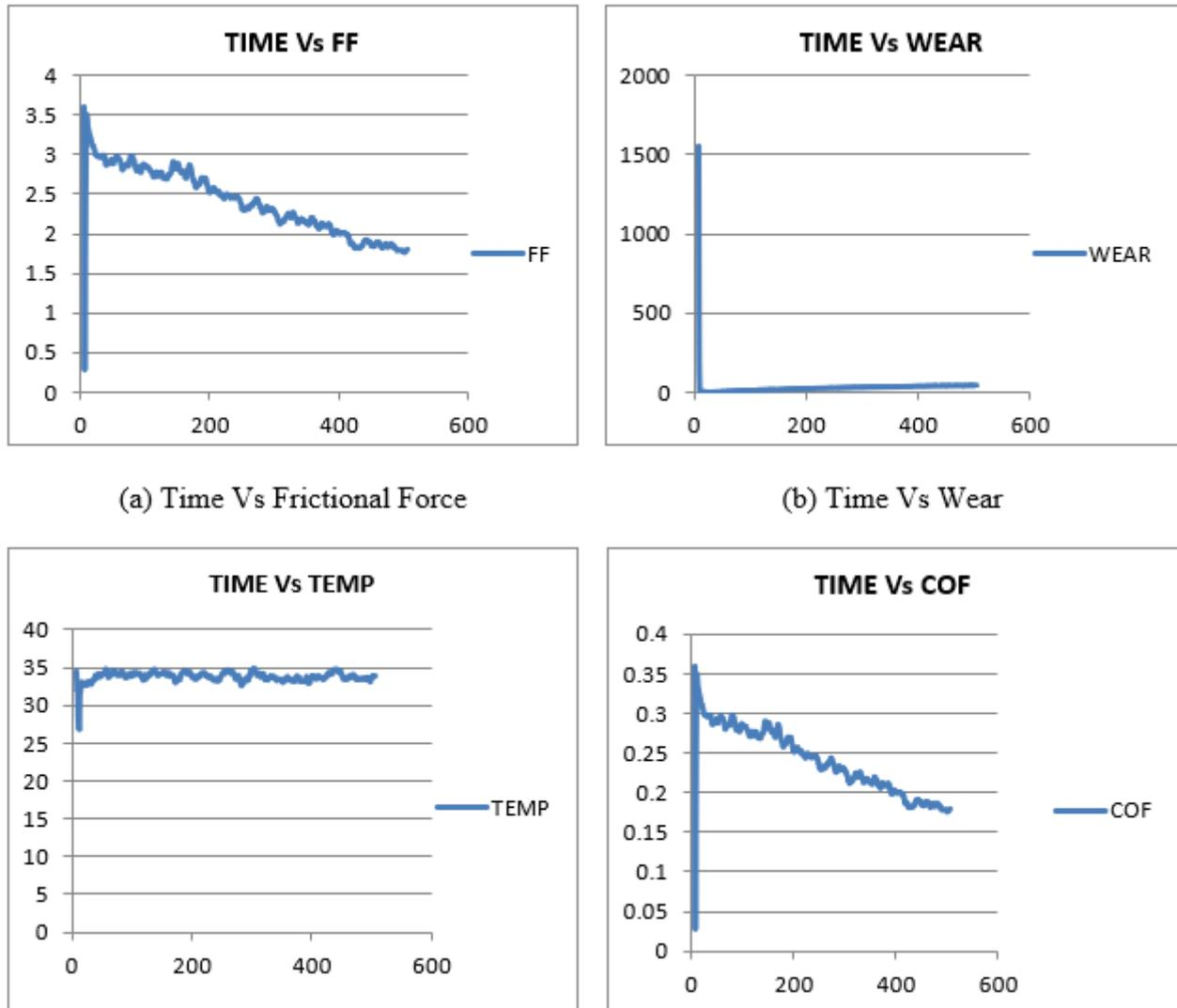
Figure 7. Time-dependent wear test results for COR sample
