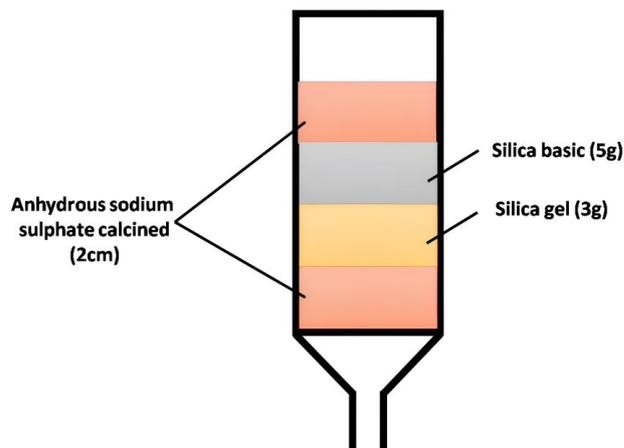
**Figure 1:** Diagram illustrating the purifying phase.
