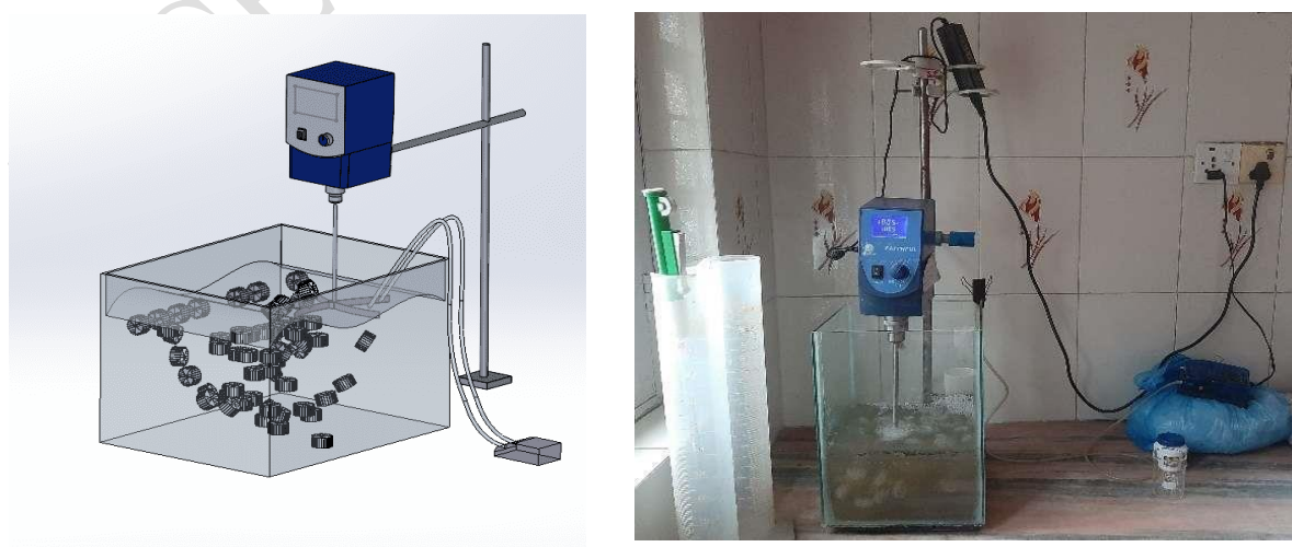
Figure 2. Experimental set-up of MBBR: A. 3D diagram of the reactor B. Actual set-up of the reactor
