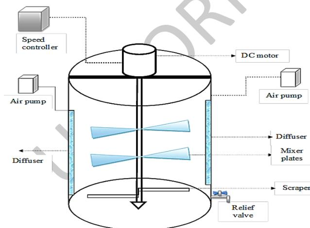
Figure 2. The aerobic reactor system
