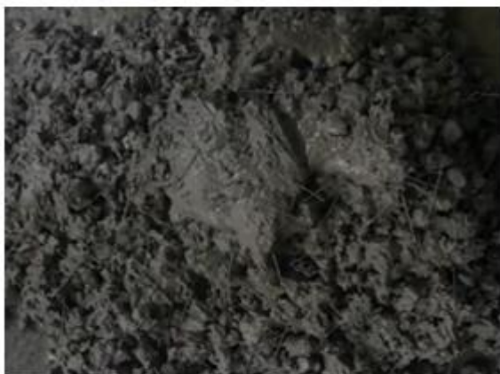
Figure 5. Crimped fiber mixed with the fresh mortar mix
