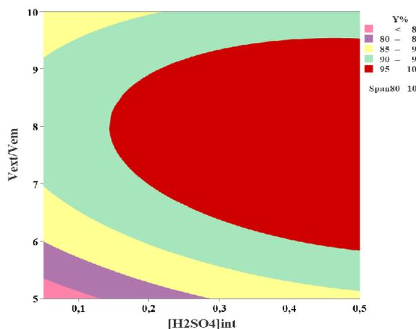
**Figure 5.** Contour area of yield as a function of  $[\text{H}_2\text{SO}_4]_{\text{int}} - V_{\text{ext}}/V_{\text{em}}$  at 10% span80.
