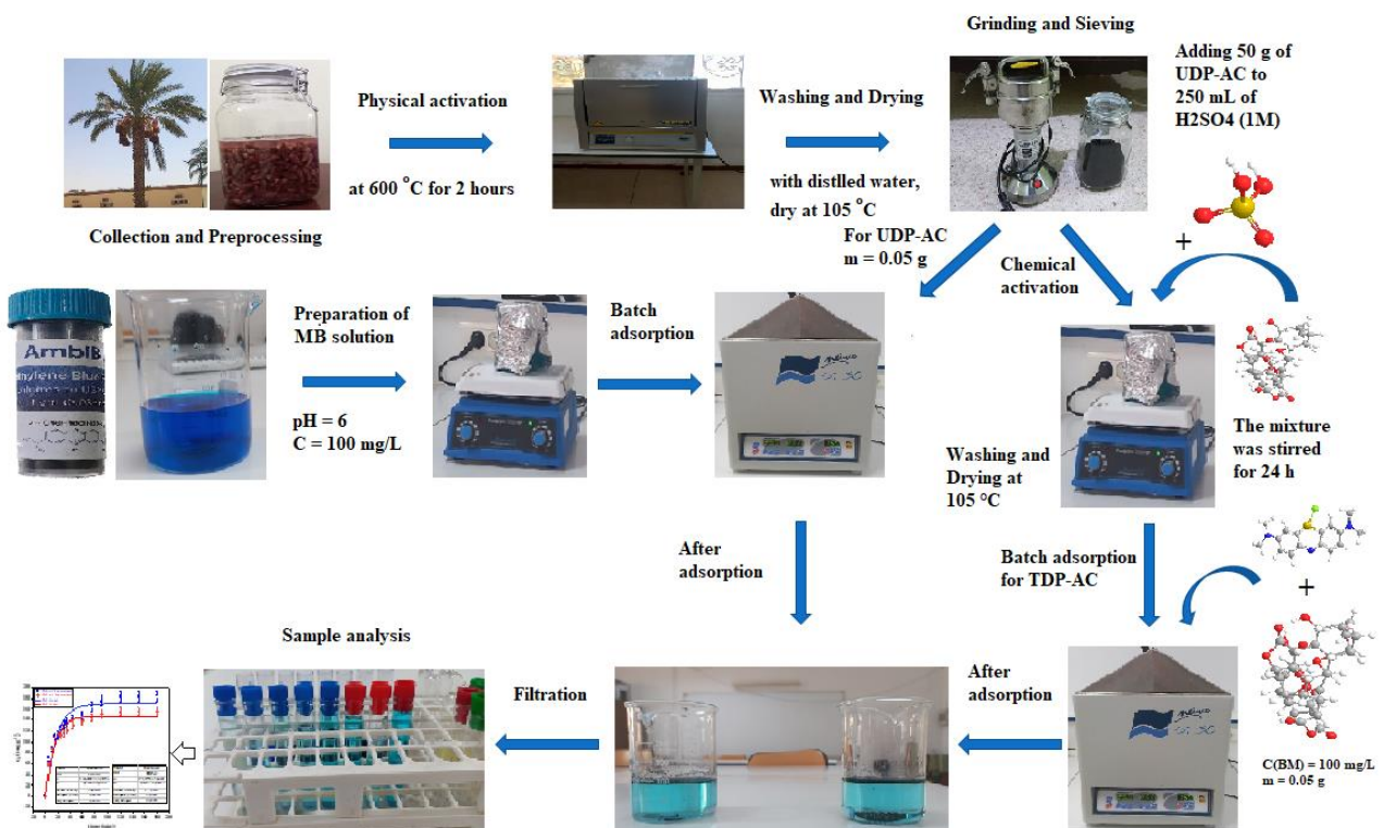
Figure 2. Stages of adsorbent material preparation and Batch adsorption process ( C_0 = 100 \text{ mg L}^{-1} , pH 6, t = 120 \text{ min} ).
