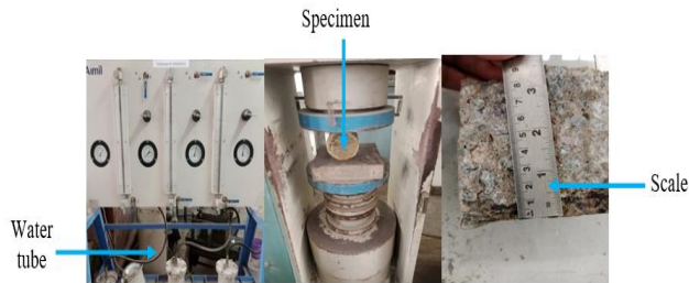
Figure 6. Test setup for Depth of penetration of water
