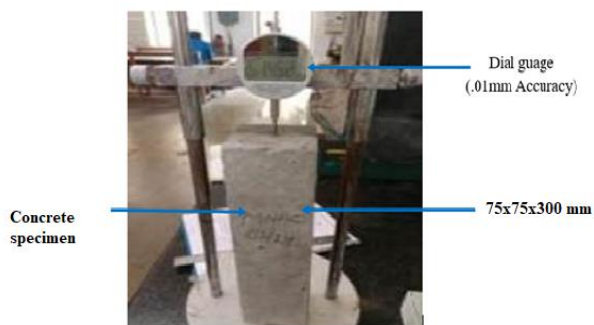
Figure 3. Test setup for Drying Shrinkage
