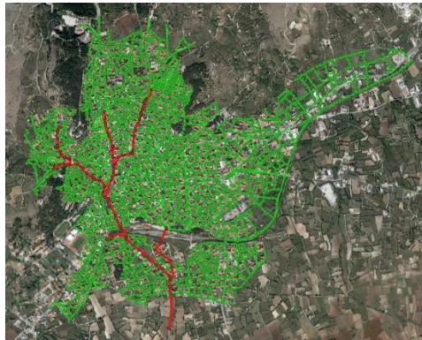
Figure 2: Sewer system of the Kozani city and the main part of the system (with red line) that is considered
