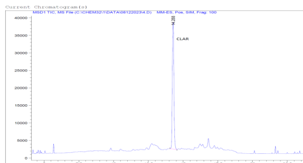
Figure 1. Standard chromatogram for antibiotic CLAR under optimum HPLC-MS conditions (10 ng/ \mu L)
