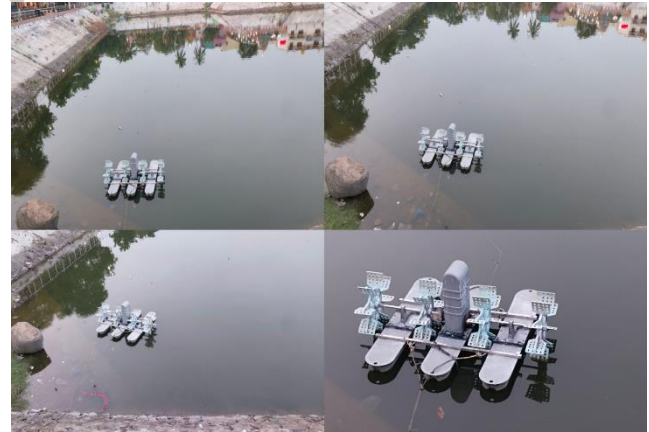
Figure 7. Aeration Floaters Device Placed in the Pond for Monitoring Oxygen levels and Water Circulation.
