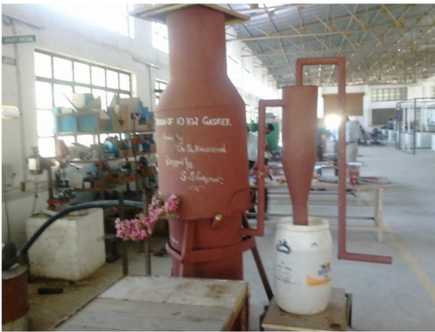
Figure 3. Fabrication setup of gasifier system.
