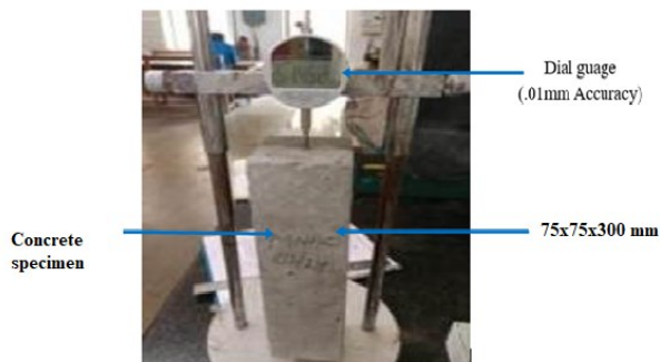
Figure 3. Test setup for Drying Shrinkage
