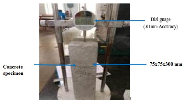
Figure 3. Test setup for Drying Shrinkage
