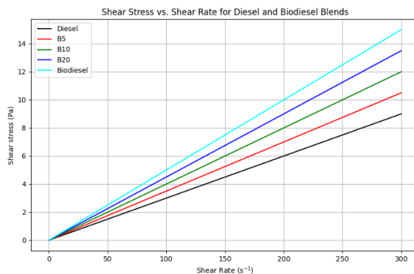
Figure 11. Shear stress curves as a function of shear rate for biodiesel (B100), its blends (B5, B10, B20), and diesel.
