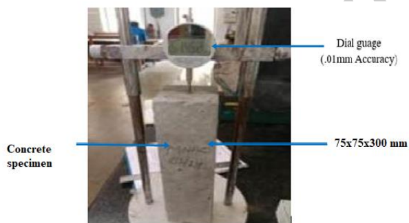
Figure 3. Test setup for Drying Shrinkage
