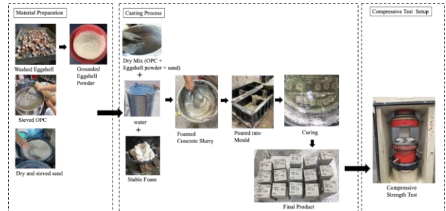
Figure 1. Process of Material, Casting and Compressive Strength Test
