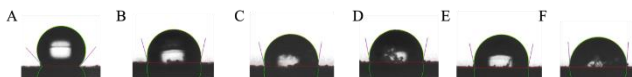
Figure 3. WCA analysis of PS after 60 h of biodegradation. (A: Control, B: Reaction system 1, C: Reaction system 2, D: Reaction system 3, E: Reaction system 4, F: Reaction system 5).
