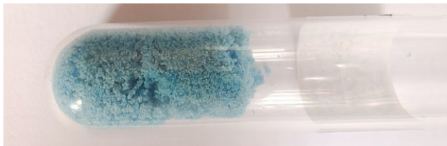
Figure 7. Solids from the tertiary freezing treatment of copper-containing electroplating wastewater
