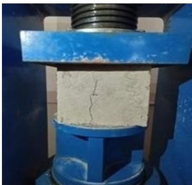
Figure 8. Compression strength characteristics test on geopolymer concrete cubes
