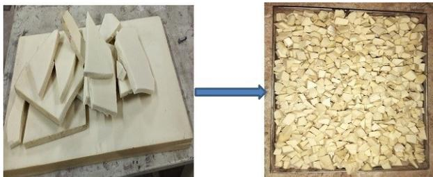
Figure 1. PUFW as coarse particles
