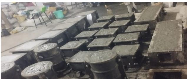
**Figure 3.** Casting of cube, cylinder and prism
