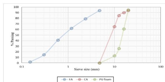
Figure 2. Particle size distribution curve of FA, CA and PUFW
