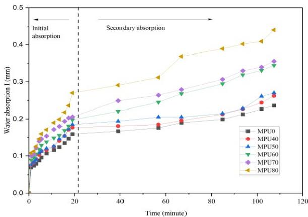
Figure 8. Water absorption by sorptivity test
