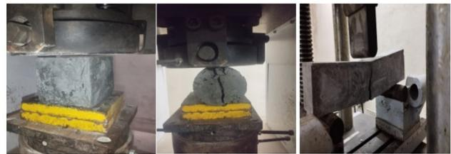
**Figure 4.** Testing of cube, cylinder and prism
