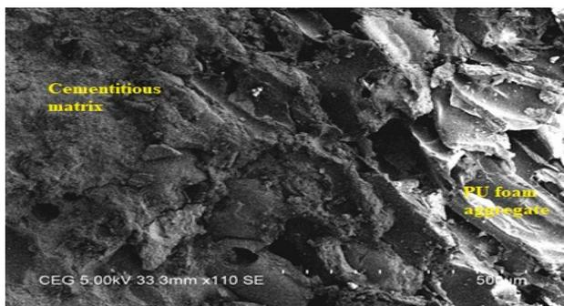
Figure 11. SEM micrograph for LWC with PUFW
