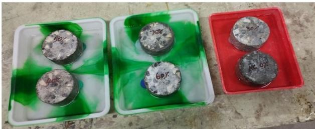
Figure 5. Water absorption by sorptivity test
