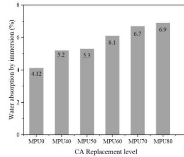
Figure 9. Water absorption by immersion
