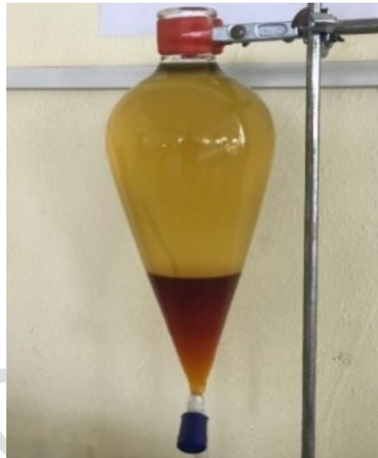
(b) Separation between glycerol and methyl ester
