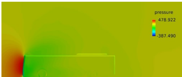
Figure 1. Pressure contour of the real bus
