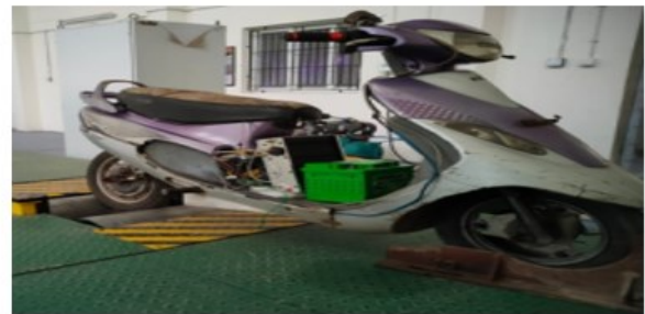
Figure 12. FC Vehicle on the Dynamometer
