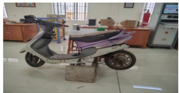
Figure 9. Fabricated Fuel Cell Based Two-Wheeler
