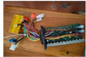
Figure 3. BLDC motor controller with specifications
