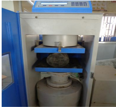
Figure 9: Split tensile strength characteristics test on geopolymer composite cylinder
