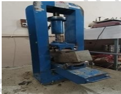
Figure 10: Flexural strength characteristics tests on geopolymer concrete prisms
