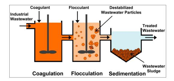
to eliminate organic compounds. Figure 1 shows the basic process of coagulation/flocculation treatment method.
