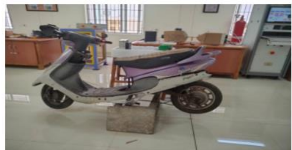
Figure 9. Fabricated Fuel Cell Based Two-Wheeler
