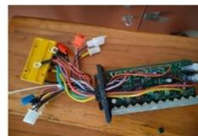
Figure 3. BLDC motor controller with specifications
