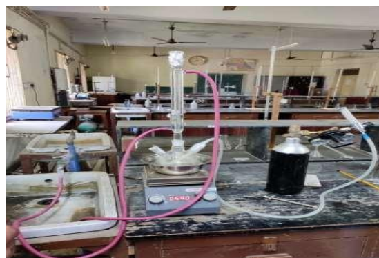
Figure 2. CO 2 Capture using Amine Bench Scale Setup
