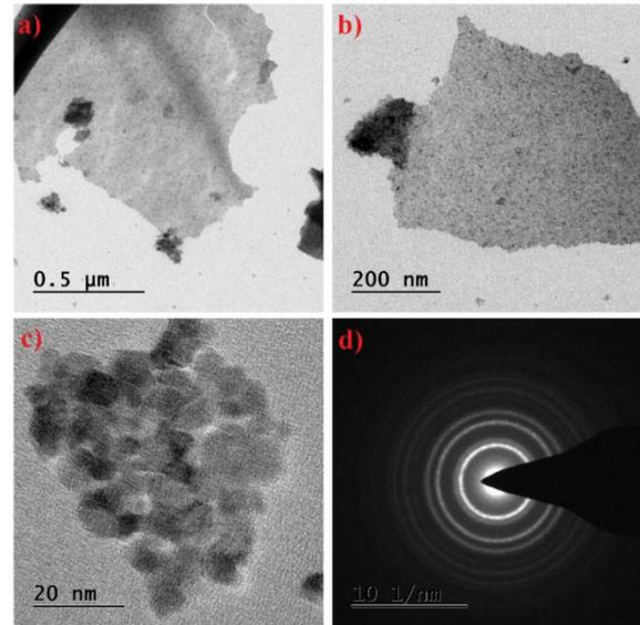
**Figure 9.** TEM image of prepared  $\text{Bi}_2\text{O}_3$  nanosheet
