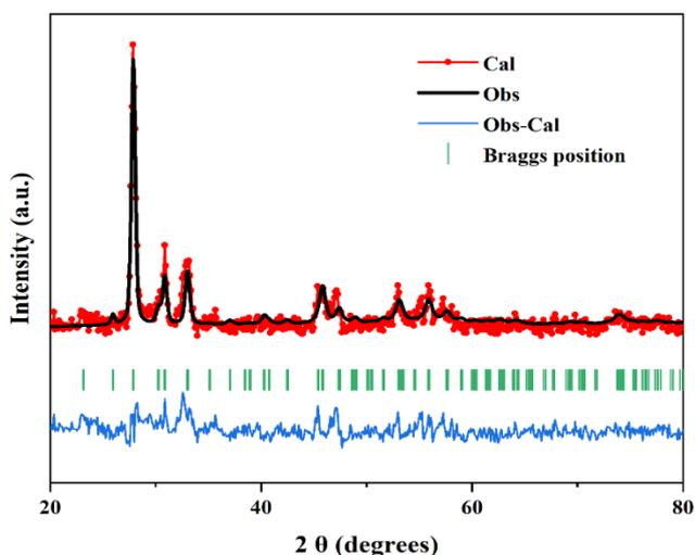
**Figure 3.** Rietveld refinement of prepared Bi<sub>2</sub>O<sub>3</sub> nanosheet
