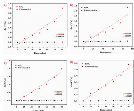
**Figure 12.** Pseudo-first-order degradation kinetics for cationic dyes: a) MG, b) Rh 6G; Anionic dyes: c) EY, d) RB
