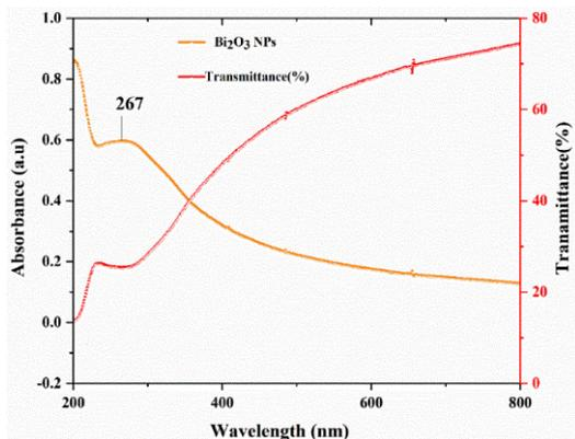
Figure 6. UV-visible spectra of Bi<sub>2</sub>O<sub>3</sub> nanosheets
