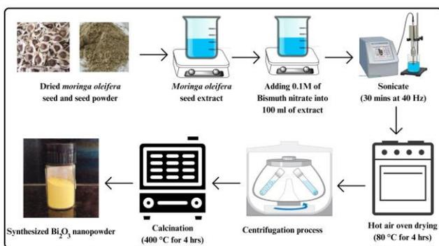
Figure 1. The  $\text{Bi}_2\text{O}_3$  nanoparticle synthesis
