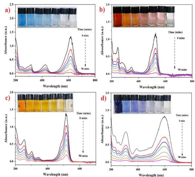
**Figure 10.** Absorbance-dye degradation graph of cationic dyes: a) MG, b) Rh 6G; Anionic dyes: c) EY, d) RB
