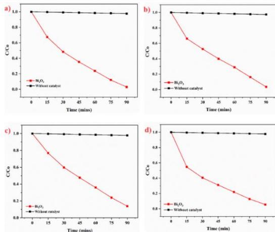
**Figure 11.** C/C<sub>0</sub> curves for cationic dyes: a) MG, b) Rh 6G; Anionic dyes: c) EY, d) RB
