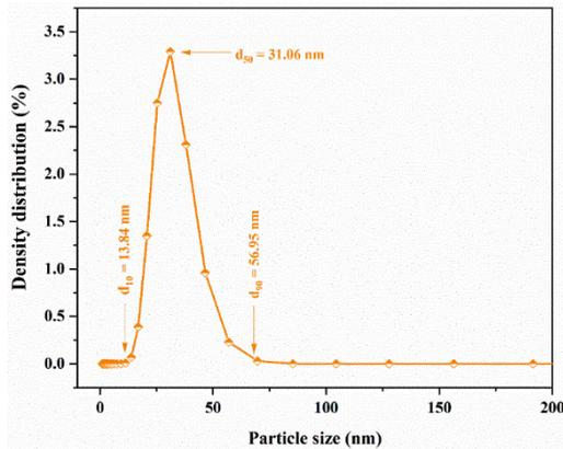
Figure 4. Particle size analysis for Bi<sub>2</sub>O<sub>3</sub> nanosheet
