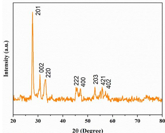
Figure 2. XRD pattern for prepared  $\text{Bi}_2\text{O}_3$  nanopowder
