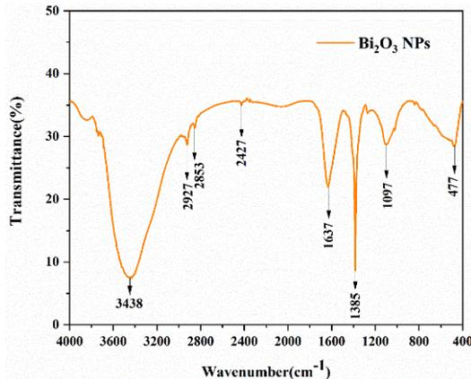
Figure 5. FTIR spectra of Bi<sub>2</sub>O<sub>3</sub> nanosheet
