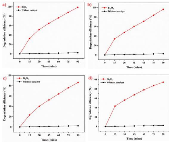
**Figure 13.** Bi<sub>2</sub>O<sub>3</sub> nanosheet degradation efficiencies against cationic dyes: a) MG, b) Rh 6G; Anionic dyes: c) EY, d) RB
