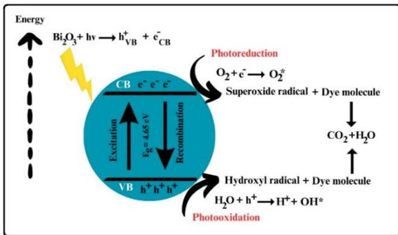
**Figure 14.** Degradation mechanism for prepared Bi<sub>2</sub>O<sub>3</sub> nanosheet
