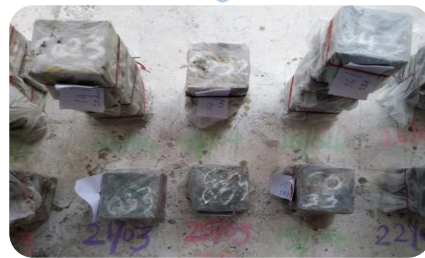
Figure 4g Specimens Demoulded - wrapped in Polythene Film and kept in Ambient curing till the day of Testing
