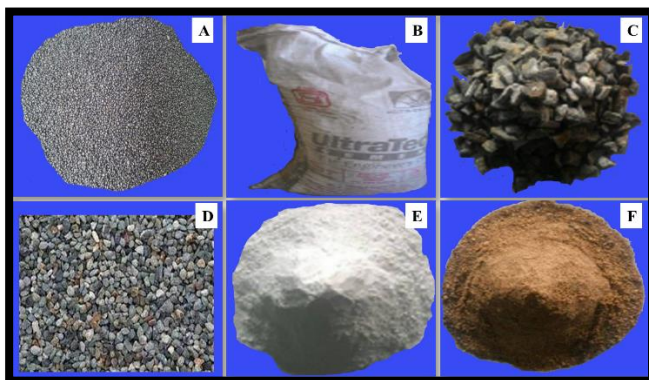
Figure 1. Materials used in current study A) NFA B) Cement C) 20mm NWA D)10mm NWA E) MWP F) MFA
