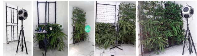
Figure 1. Some measurement documentation with various numbers of biowall modules
