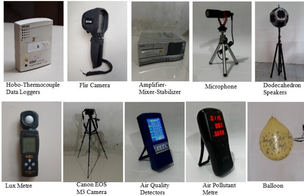
Figure 4. The main instruments for thermal, audial, visual, and respiratory measurements
