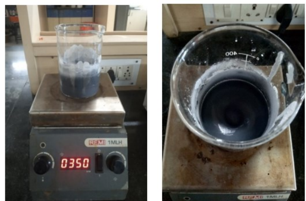
Figure 14. Dispersion of NCP char using magnetic stirrer
