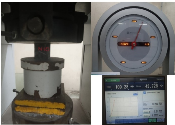
Figure 4. Test setup of CTM for compressive strength
